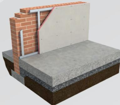
5. Fix SR/TB-MF to the frame at 300mm centres using appropriate fixings eg. drywall screws, at least 12mm in from the board edge. The fixings should penetrate at least 25mm into the timber batten. Fixings should be thermally broken where possible.
