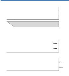
NVFB -Product width across cavity from 281mm-455mm wide fixed using 2 High Performance (HP) 328mm brackets.
