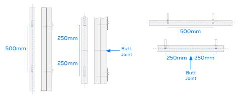
Push the cavity barrier onto the bracket spike, the brackets should impale the NVFB to approximately mid barrier depth and must not protrude through the face of the cavity barrier, remembering to allow for the final compression against the outer substrate also. The cavity barrier should be pushed fully onto the bracket spike and sit flush with the substrate, at the rear of the cavity barrier, ensuring that there are no gaps behind the cavity barrier.
