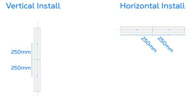
NVFB - Product width across cavity from 81mm up to 95mm, fixed using 2 multi purpose (MP) 65mm brackets.
