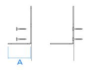
For cavity barriers 81mm-95mm wide (across cavity) use 2 MP brackets and the 65mm long spike (A). To secure the bracket use 5mm  $\emptyset$  stainless steel screws, with a maximum head diameter of 13mm and with a length and type suitable for the substrate. Ensure that the screw head sits as flush as possible with the substrate so that the NVFB sits tight against the substrate leaving no gaps. Fix through both of the fixing holes.
