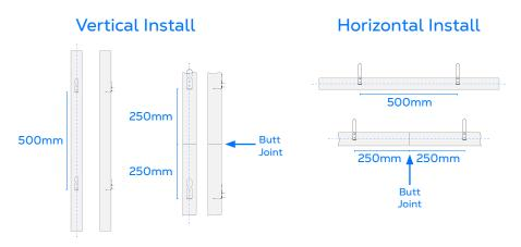
Push the cavity barrier onto the bracket spike, the brackets should impale the NVFB to approximately mid barrier depth and must not protrude through the face of the cavity barrier, remembering to allow for the final compression against the outer substrate also. The cavity barrier should be pushed fully onto the bracket spike and sit flush with the substrate, at the rear of the cavity barrier, ensuring that there are no gaps behind the cavity barrier.
