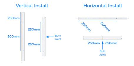
Where sections of cavity barrier are less than 1 linear meter in length, ensure that face fixings are positioned at a maximum 250mm from each end. For cut sections of cavity barrier less than or equal to 500mm in length only one fixing is required.
