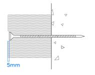
Use stainless steel countersunk head screws, with a maximum head diameter of 11.5mm and with a length suitable for the cavity barrier and the substrate. Ensure that the countersunk screw head does fully penetrate the face of the cavity barrier, the screw head should sit at least 5mm behind the face of the cavity barrier. Care should be taken not to compress the surface more than 10mm as this may effect the performance of the cavity barrier.
