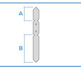
MP brackets are supplied with 2 fixing spikes, one spike is 65mm long (A), the other is 160mm long (B), with a central section for securing the bracket to the substrate. The compression allowed for is 5mm, care should be taken to ensure that the end of the bracket will not come into contact with the outer substrate when compression is applied to the NVFB.
