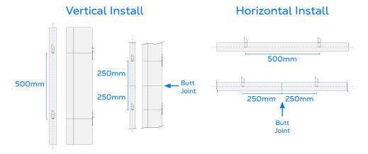
Push the cavity barrier onto the bracket spike, the brackets should impale the NVFB to approximately mid barrier depth and must not protrude through the face of the cavity barrier, remembering to allow for the final compression against the outer substrate also. The cavity barrier should be pushed fully onto the bracket spike and sit flush with the substrate, at the rear of the cavity barrier, ensuring that there are no gaps behind the cavity barrier.
