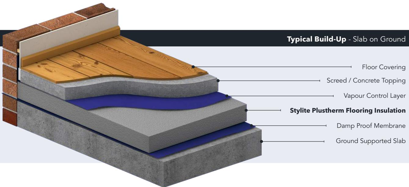
**Typical Build-Up - Slab on Ground**
