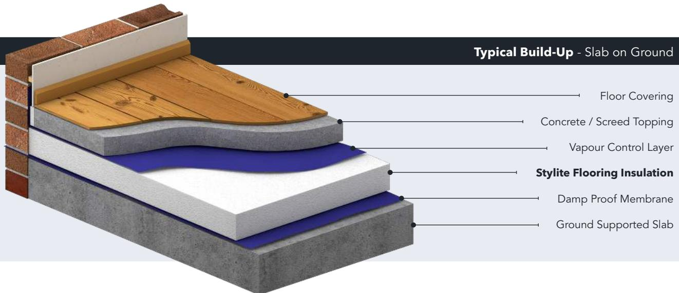
Typical Build-Up - Slab on Ground
