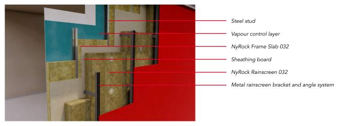
Steel Frame System with Brick Outer
