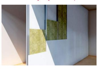
Studs: 50mm metal 'C 'studs at 600mm Centres
