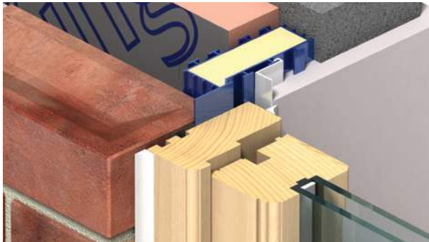
Figure 23: Kingspan Thermabate® in Position with Reveal Clip Engaged behind Window Frame
