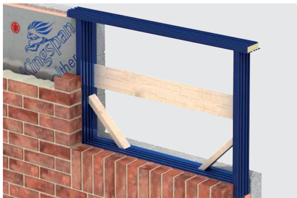
Figure 18: Kingspan Thermabate® Built-in as the Wall is being Constructed
