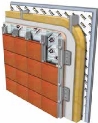
SFS with rainscreen cladding
